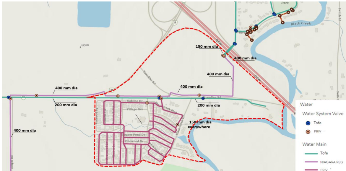
Figure 2-2 - Existing Municipal Water System
