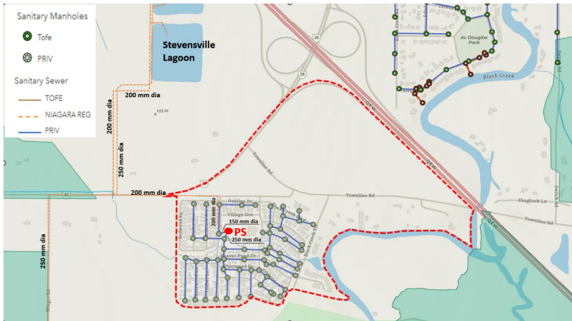
Figure 2-3 - Existing Sanitary System
